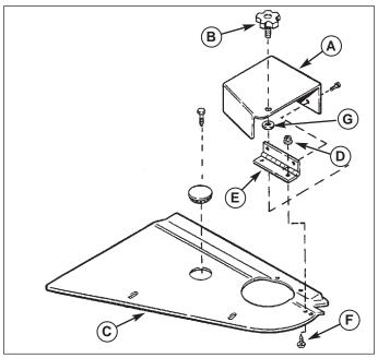
Figure 2. Assemble the New Cover
